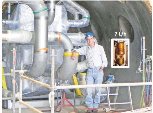
Figure 5: Inside the cold box of the 8000 l/h helium liquefier (near me, in the white frame, one of my old 7 l/h heat exchanger batteries at the same scale!)
