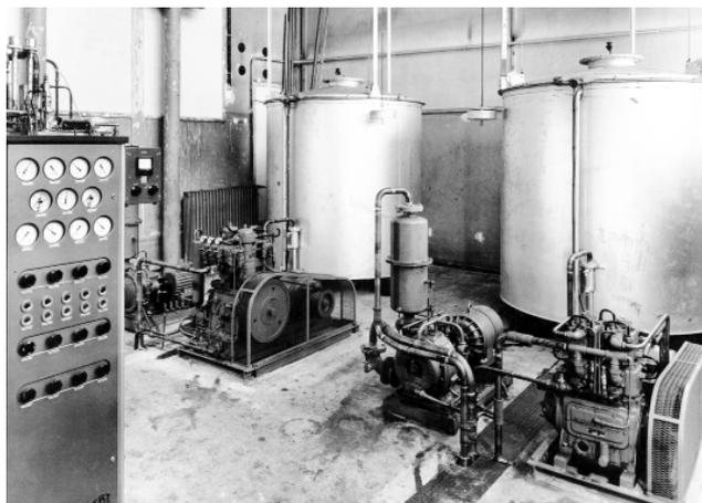
**Figure 3: The 7 L/h helium liquefier (from left: cold box helium compressor, helium gas holder, nitrogen vacuum pump, hydrogen gas holder, hydrogen compressor)**
